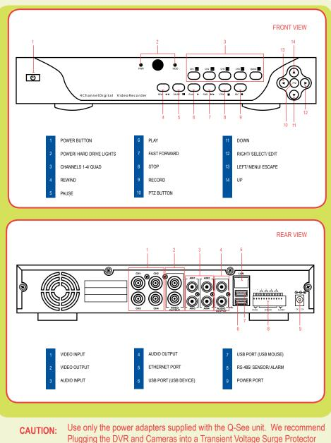
(UL-449 Rating)\* 330 or lower clamping voltage, Joule rating 400.
